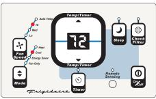
Note: Tap or hold either up(^) or down(v) button until the desired temperature is seen on display. This temperature will be automatically maintained anywhere between 60F (16°C) and 90F (32°C) for cooling mode. The Temperature will be automatically maintained anywhere between 55F (13°C) and 80F (27°C) for heating mode. If you want the display to read the actual room temperature, "FAN SEE ONLY MODE".
